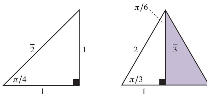
Triangles for determining special values of the trigonometric functions.
