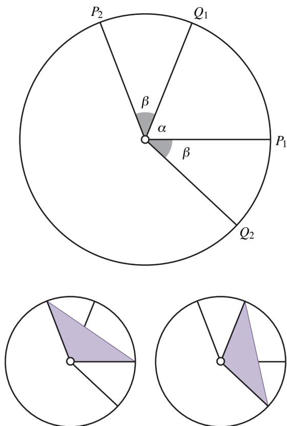
The setup for the derivation of the Addition Formula for Cosine. The key is that the distance from  $P_1$  to  $P_2$  is the same as the distance from  $Q_1$  to  $Q_2$ .
